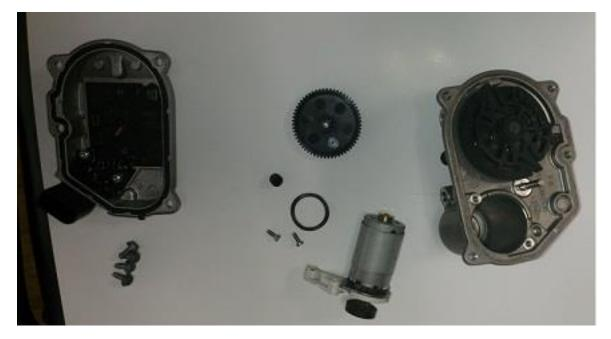
Step 4. Take the top part (the one with the electronic connector). Disconnect the unnecessary wires. Then, using the provided schematics, you will need to solder the new wires onto the free slots.
