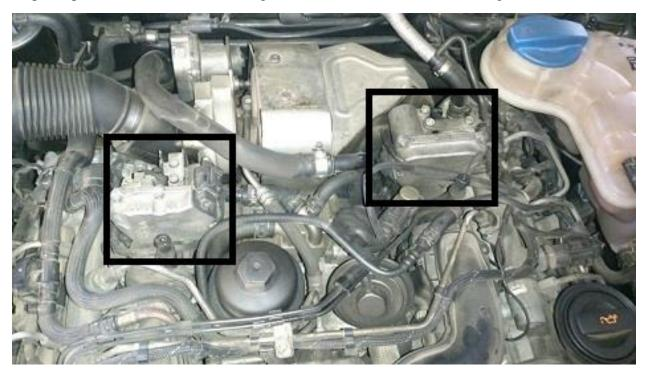
The inlet manifold flap motors are clearly marked. Undo the bolts and remove the flap connector. Remove them from the engine bay.
