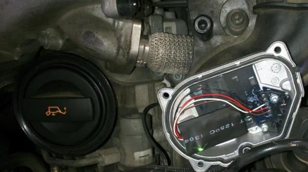
Then use the free space where the motor used to be to accommodate the emulator.
