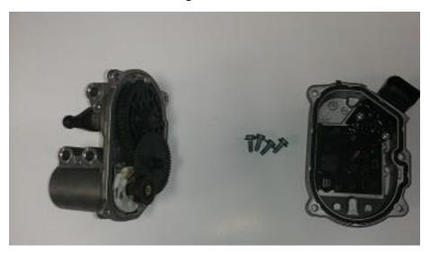
Step 3. Further disassembly is needed. You have to take the motor out by removing the little plastic cap that holds the rotor in place. Later you can remove the rotor which then lets you remove the motor itself by unscrewing two bolts.
